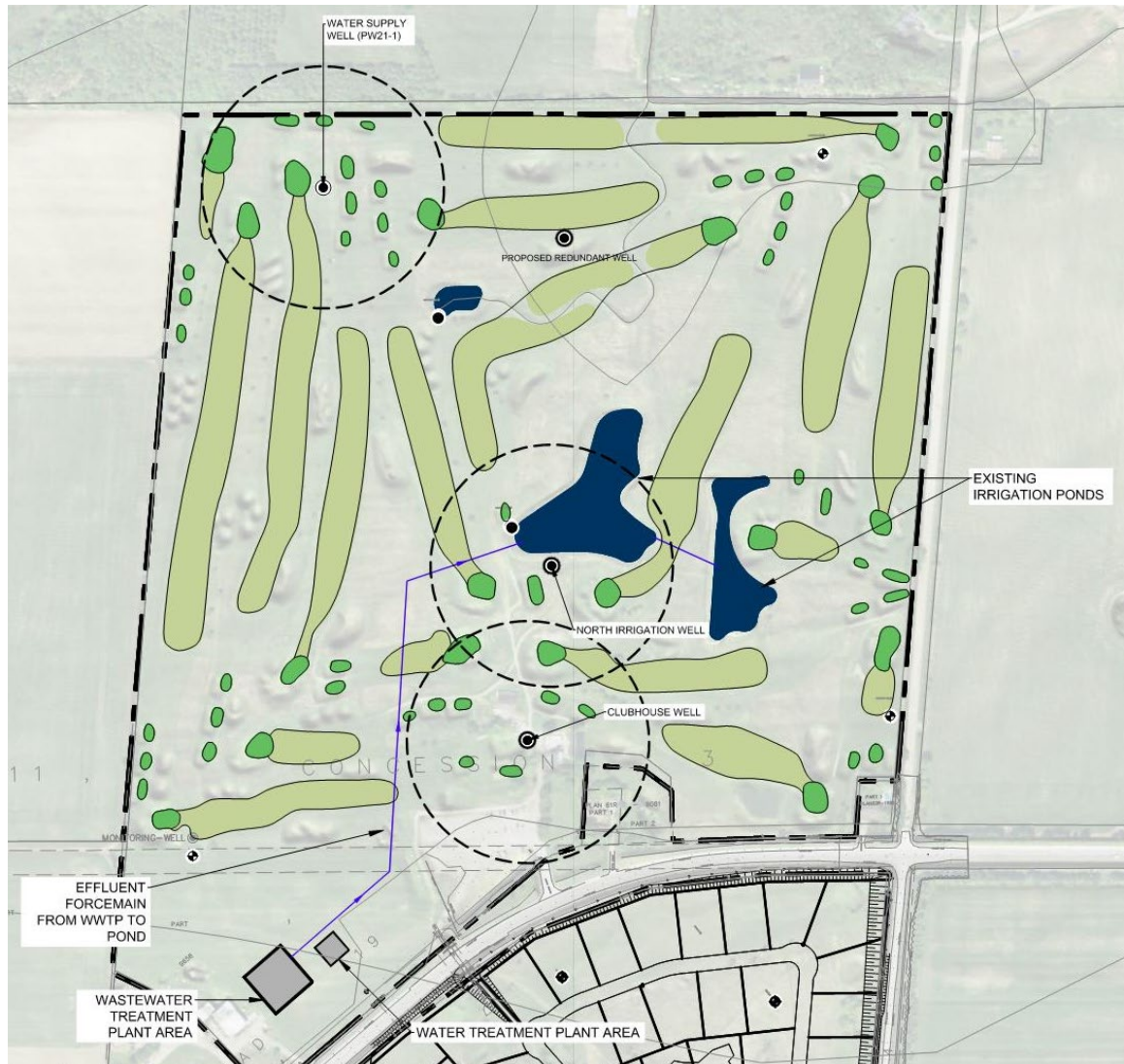
Figure 5-6: Alternative Solution 5 – Wastewater Servicing
